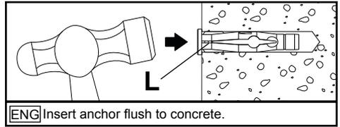
**ENG** Insert anchor flush to concrete.
