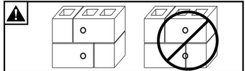
ENG Do not drill into mortar joints.
