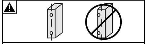
**ENG** Mounting hole must center on stud.
