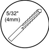
**ENG** Drill mounting holes into supporting surface (2.5" (64 mm) minimum depth required).
